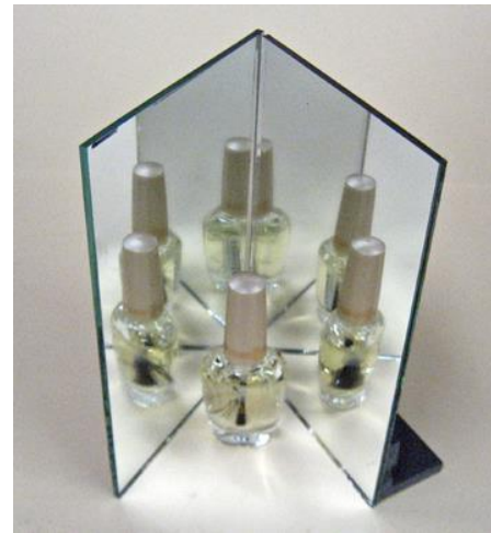
Two mirrors at a 60° angle
