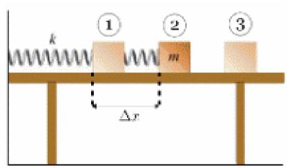
Assume that the spring is being held in place by an external force until time 1, which is the instant that this force is removed from the mass. At time 1 the system begins with exactly **6 J** of energy. Time 2 is the moment when the spring and the mass lose contact. Time 3 is the final position of the mass after it has stopped moving along the table.
