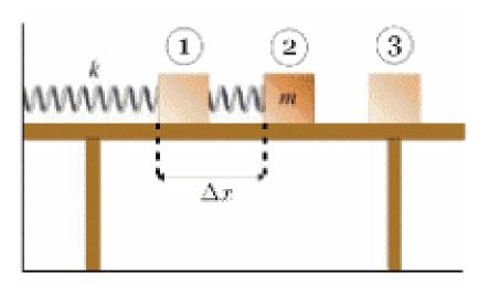
Assume that the spring is being held in place by an external force until time 1, which is the instant that this force is removed from the mass (this is the moment before the mass starts moving due to the expansion of the spring). At time 1 the system begins with exactly **6 J** of energy.
