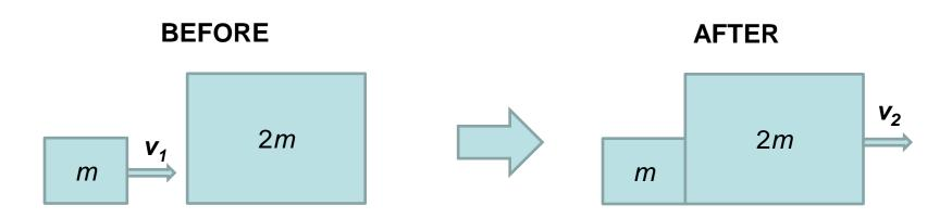
Initially, the kinetic energy of the system is:  $E_{K_1} = \frac{1}{2}mv_1^2$
