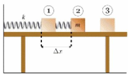
Assume that the spring is being held in place by an external force until time 1, which is the instant that this force is removed from the mass. At time 1 the system begins with exactly **6 J** of energy. Time 2 is the moment when the spring and the mass lose contact (this is when the spring reaches its equilibrium length).
