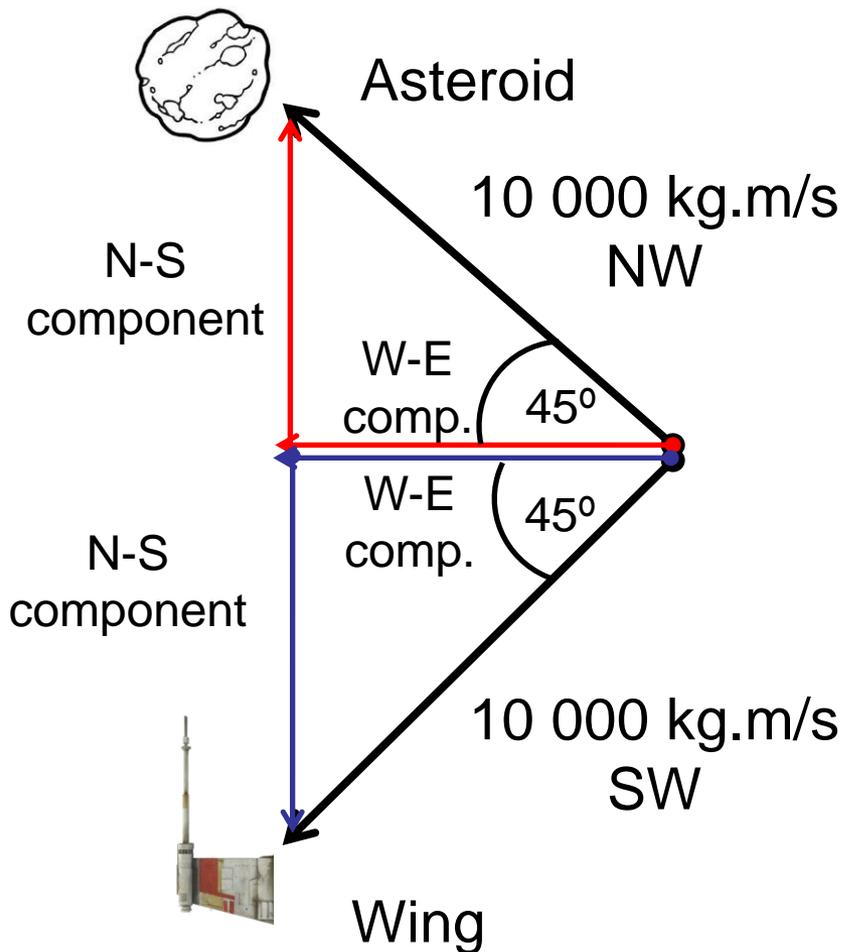
We can see from the diagram that since the magnitude of each of the momentum vectors is equal, then their West-East components and North-South components must also be of equal magnitude.
