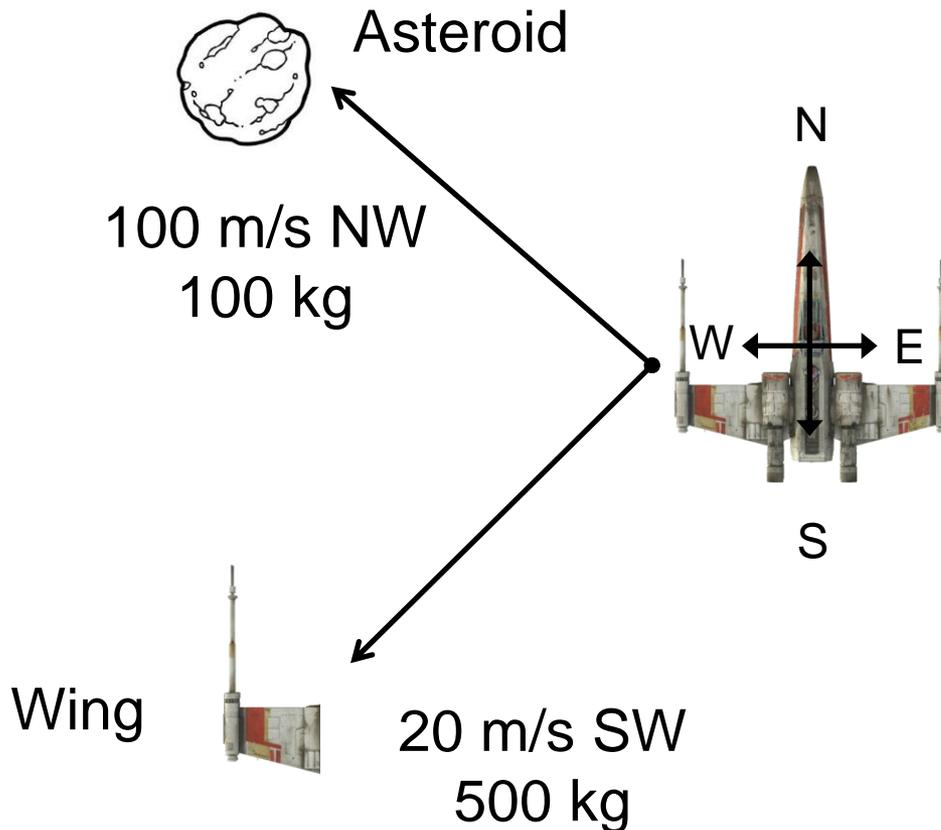
We can calculate the momentum of both the wing and the asteroid using the equation  $\mathbf{p} = m\mathbf{v}$ :
