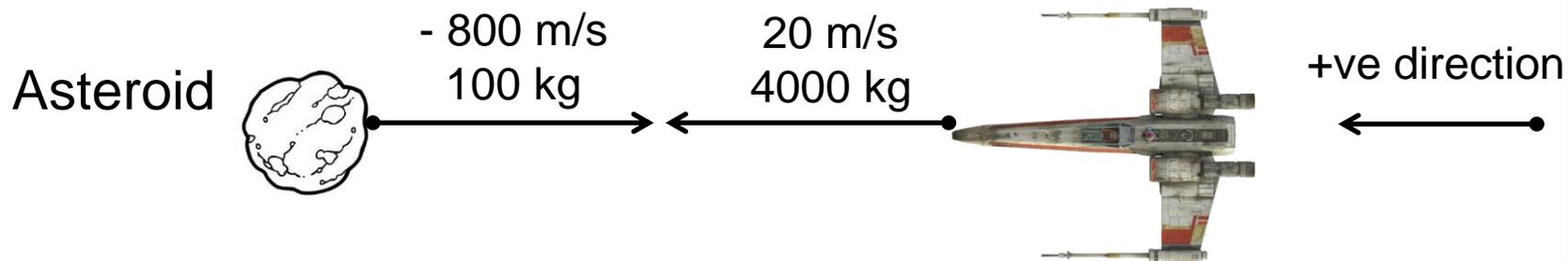
We can then calculate the momentum of both the asteroid and the ship using the equation  $\mathbf{p} = m\mathbf{v}$ :
