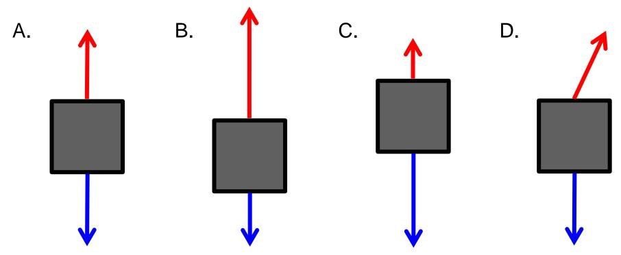
**Note:** The grey square represents the rocket, the red arrow represents thrust and the blue arrow represents gravity (weight).
