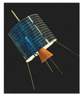
These satellites must be able to withstand the shock of a launch into orbit at a speed greater than 28 000 km/h. Satellites must be small and made of lightweight materials in order to remain intact in an environment of high radiation and extreme temperature. Many satellites have an operational lifetime of up to 20 years.
