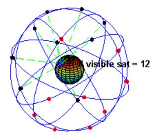
A visual example of a 24 satellite GPS constellation in motion with the Earth rotating. Notice how the number of **satellites in view** from a given point on the Earth's surface, in this example at 45°N, changes with time.
